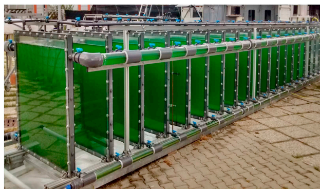
Fig. 10. The flat panel PhotoBioReactor (PBR) system (maximum working volume 1300 L) is composed of 20 vertical parallel plates 50 L, 1150 × 1150 × 50 mm ( W \times H \times D ), in direct communication with each other, left. Daily variation of maximum quantum efficiency of PSII photochemistry ( F_v/F_m ) and effective photochemical quantum yield of PSII ( \Delta F/F_m' ) right. Data are shown as mean \pm SD, n = 3 .
